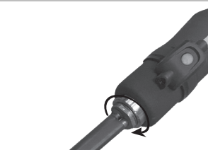
Tightening torque max = 7N
